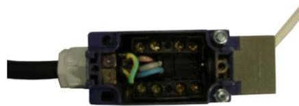
**NB: if the winch is monoblock (winch + sécurichute), replace the cable from the top limit switch by a cable with 1m length.**
